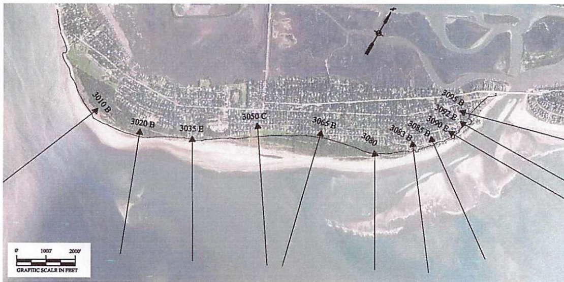
Figure 2. 2015 aerial photo illustrating the eleven (11) beach profile lines and corresponding SCDHEC-OCRM Monuments on Sullivan's Island. The solid black line running parallel to the shoreline through the dunes is the OCRM Baseline.
