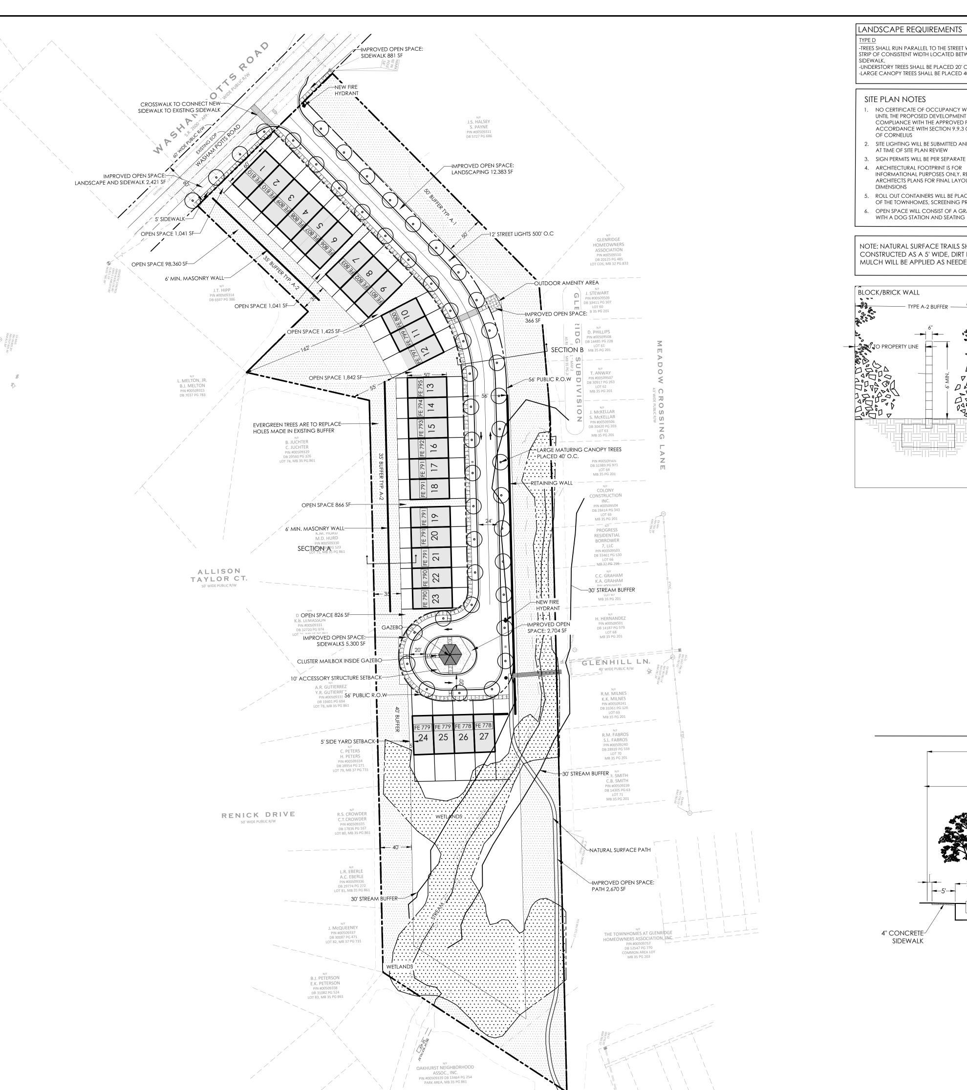
LANDSCAPE REQUIREMENTS -TREES SHALL RUN PARALLEL TO THE STREET WITHIN A PLANTING STRIP OF CONSISTENT WIDTH LOCATED BETWEEN THE CURB AND -UNDERSTORY TREES SHALL BE PLACED 20' O.C. -LARGE CANOPY TREES SHALL BE PLACED 40' O.C.
