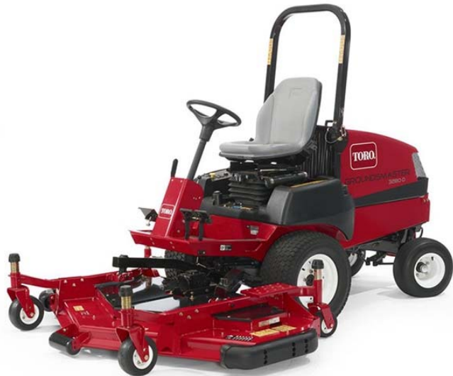
Groundsmaster 3280 – used to cut rough, thick vegetation (small trees, shrubs)
